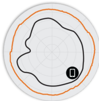
Figure 3. T750 5GHz Azimuth Antenna Patterns
