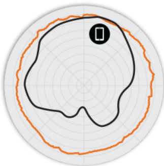
Figure 2. T750 2.4GHz Azimuth Antenna Patterns
