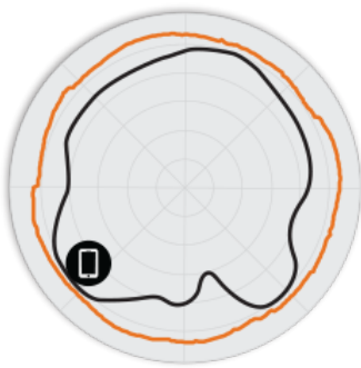
Figure 2. T350c/d 2.4GHz Azimuth Antenna Patterns
