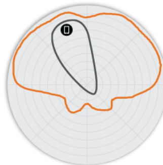
Figure 4. T750 2.4GHz Elevation Antenna Patterns
