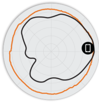
Figure 3. T350c/d 5GHz Azimuth Antenna Patterns
