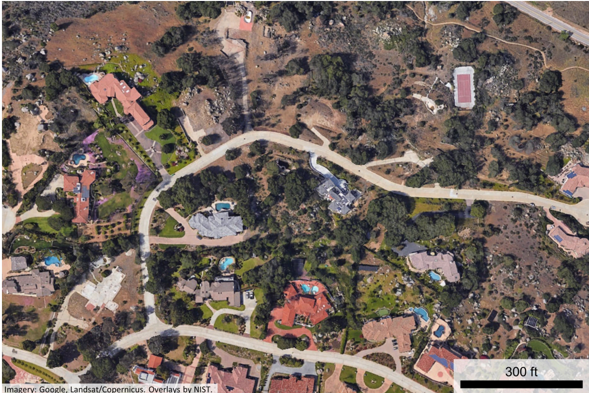
Figure 5. WUI Type 6: Low Density Intermix, The Trails, Rancho Bernardo, CA. Note irrigated lawns, long paved driveways, pools and tennis courts. Some structure-to-structure distances are representative of Moderate Density Intermix (lower part of image). Also note limited high density non-irrigated vegetative loading.
