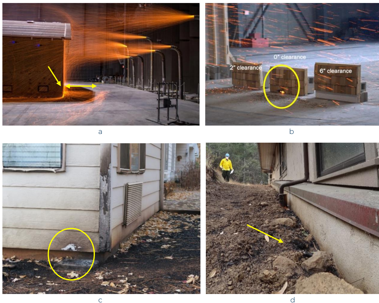
Figure 4. Ember accumulation at the base of the wall causing ignition (a and b) at the IBHS Research Center, (c) in the post-Camp Fire (2018) investigation in Butte County, California, and (d) at the base of a wall in the Glass Fire (2020) in Napa and Sonoma Counties, California, which did not have the opportunity to grow because of a noncombustible vertical clearance.
