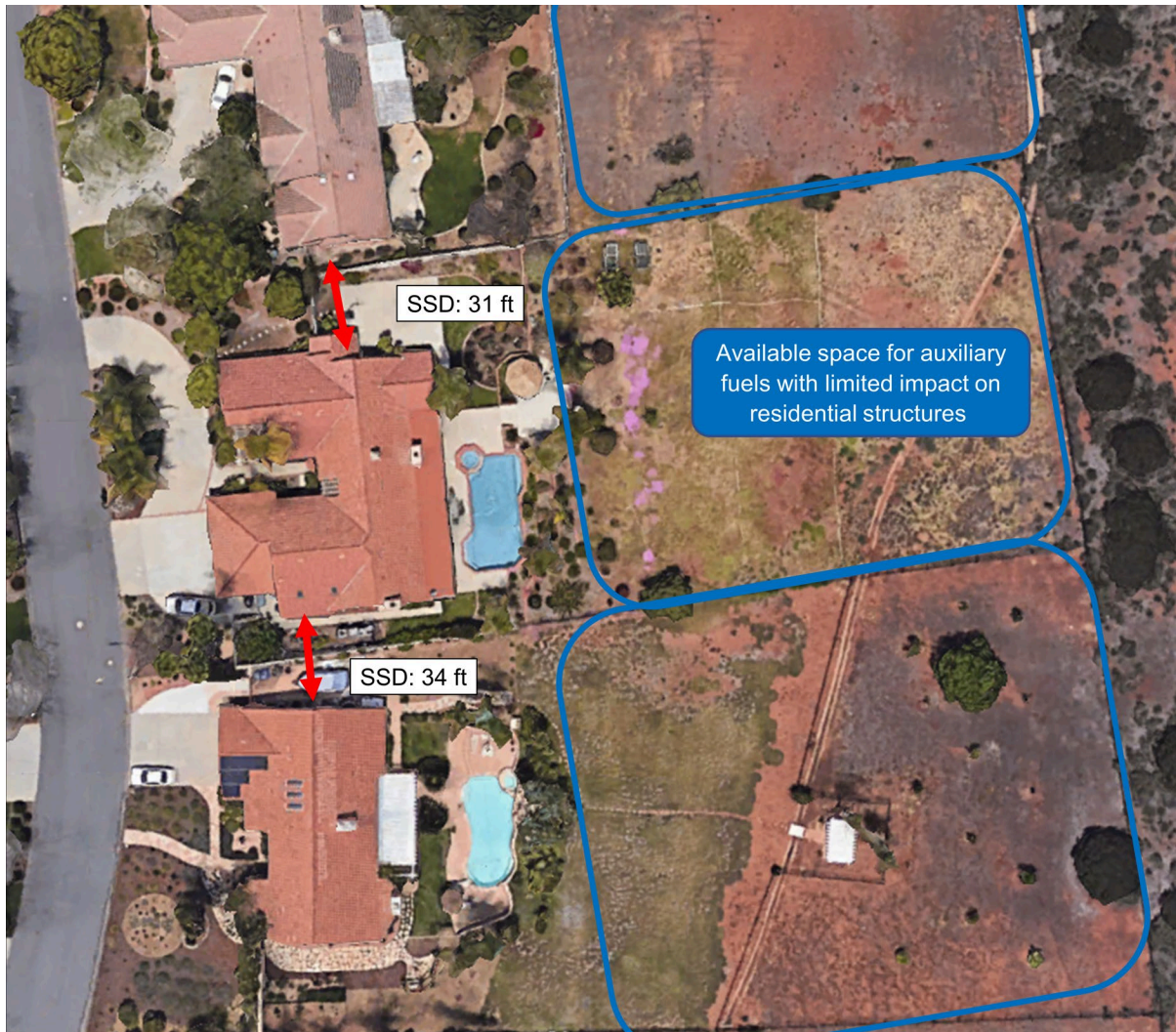
Figure 19. Scenario C, WUI Type 4 or Type 6. While the structures are placed on large parcels with extensive backyards, the primary structures are very large with considerably smaller SSD. Selective hardening may be required in this scenario despite the large parcels.
