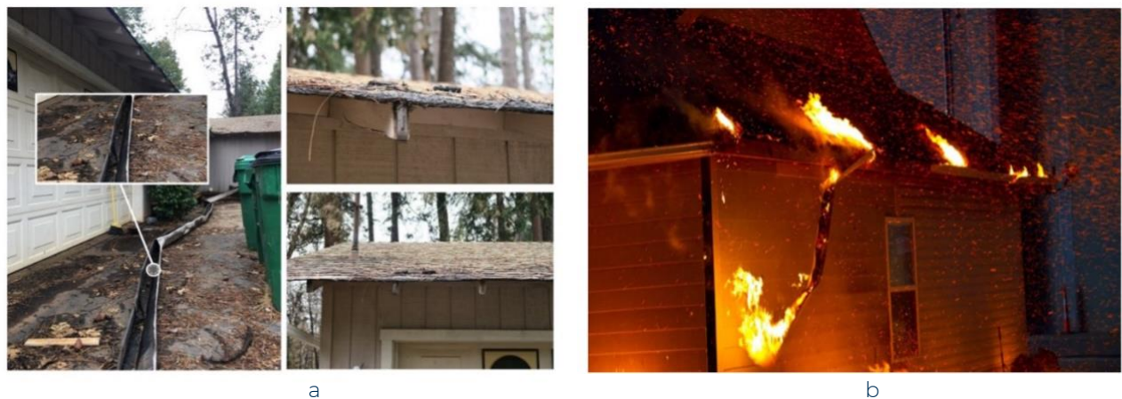
Figure 1. Direct flame contact to the edge of the roof caused by ignited debris in the gutters during ember storms (a) in the Camp Fire (2018) in Butte County, California (home defended by first responders), and (b) a vinyl gutter melts off a house during testing at the IBHS Research Center.
