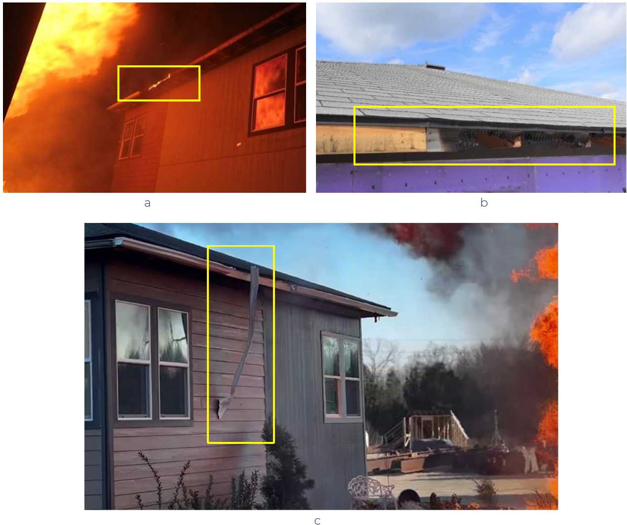
Figure 2. A noncombustible gutter can provide protection for the fascia board if a metal drip edge is not installed. (a) shows fascia board ignition during the experiment and (b) shows the fascia board condition after the test. In (c), a vinyl gutter deformed due to radiant heat/intermittent flame contact and fell off.
