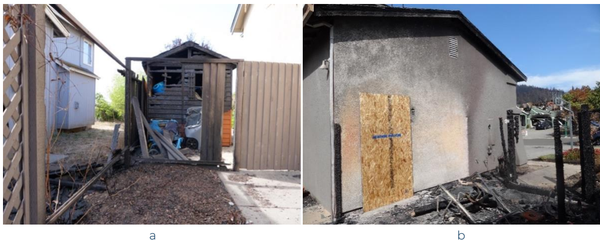
Figure 8. Example of a shed damaging the main structure on a parcel in the Glass Fire (2020) in Napa and Sonoma Counties, California. In photo (a), a shed was about 6 ft away from the main structure (suppressed by first responders and the homeowner). In photo (b), an attached outbuilding completely burned and damaged the main structure (suppressed by first responders).
