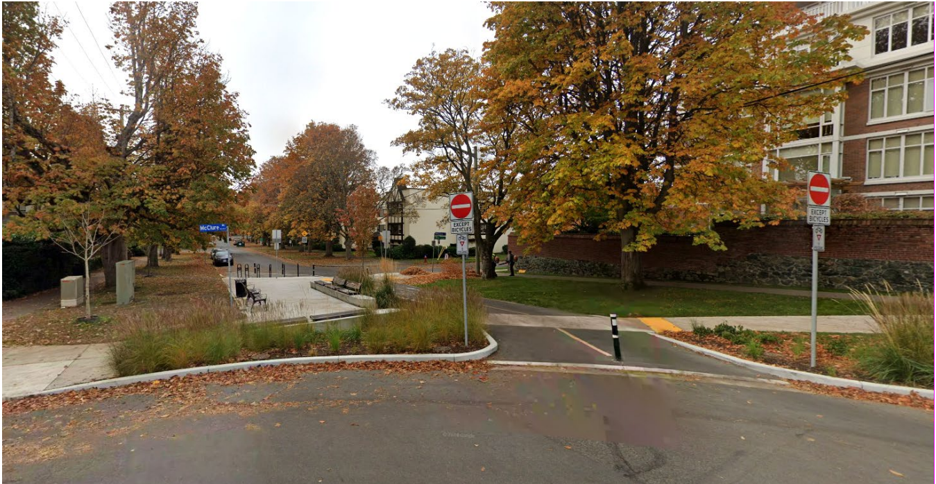
Figure 5.30 Street closed to vehicles and converted into a plaza with landscaped seating with bicycle and emergency vehicle pass-through at Vancouver Street and McClure Street, Victoria, BC. Google maps , November 2022.
