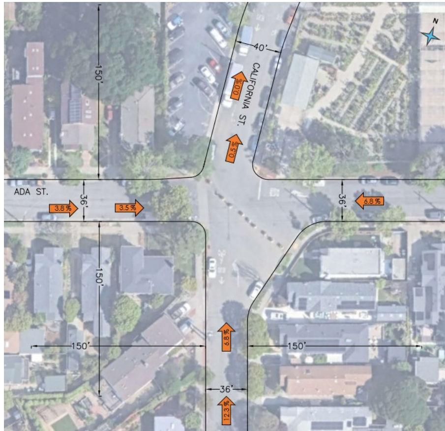
Figure 2. Roadway Grades / Slopes
