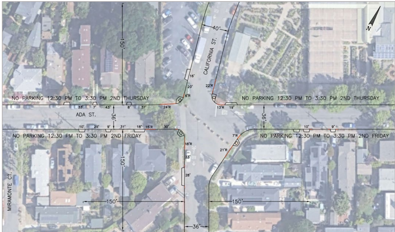
Figure 1. California Street and Ada St intersection measurements
